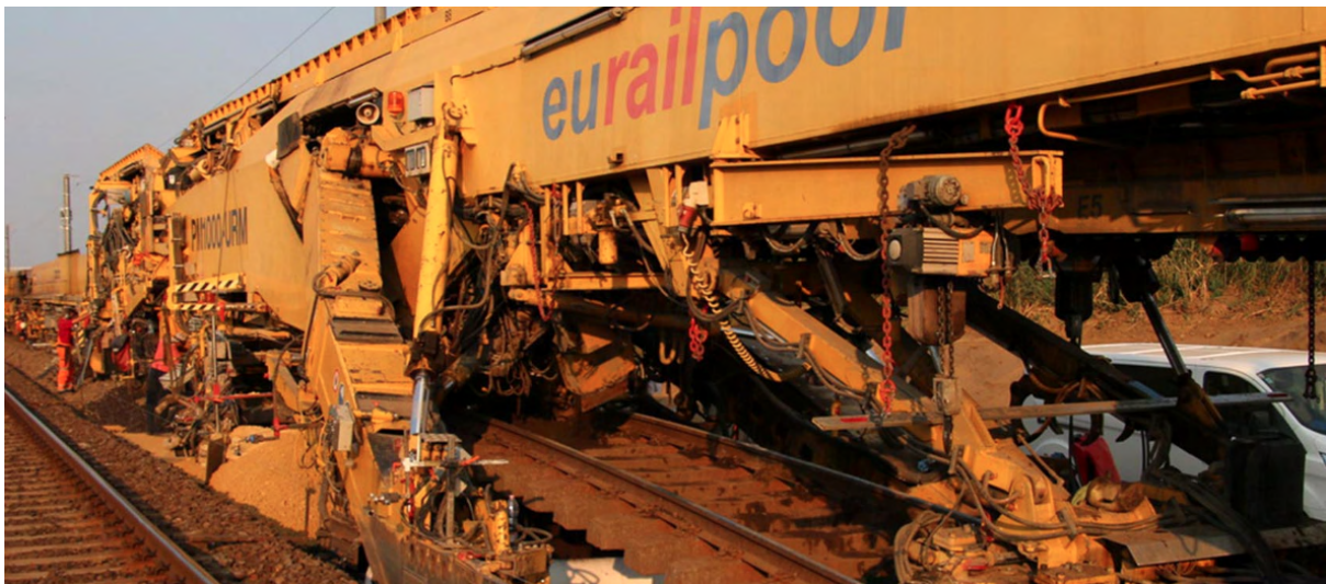
Figure 20: a shoulder ballast cleaning machine, also known as a ballast cleaner, can rehabilitate the ballast with a recycling rate of up to 100% (Eurailpool n.d.). The type of cleaner shown in this picture, the PM1000 URM is used in Dutch rail maintenance works by the company Swietelsky (Swietelsky 2019).
