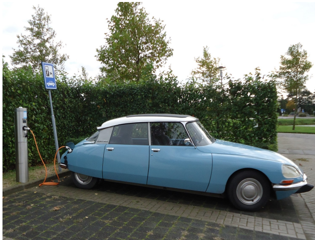
Figure 5.3: A 1972 (48-year old) Citroen DS retrofitted with an electric drivetrain ( Reins, 2019 ).
